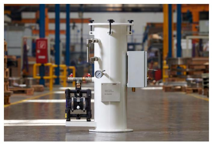
After the Turbulo Sludge Buoy's installation, the Turbulo SolidMaster serves as filtration system which precedes the oily water separator (OWS) and mechanically removes suspended solids in the bilge water. Doing this before running the bilge water through the separator helps avoid the formation of suspensions and thereby extends the lifetime of the – more expensive – separation elements of the OWS.
